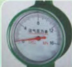
Biogas Pressure Gauge
